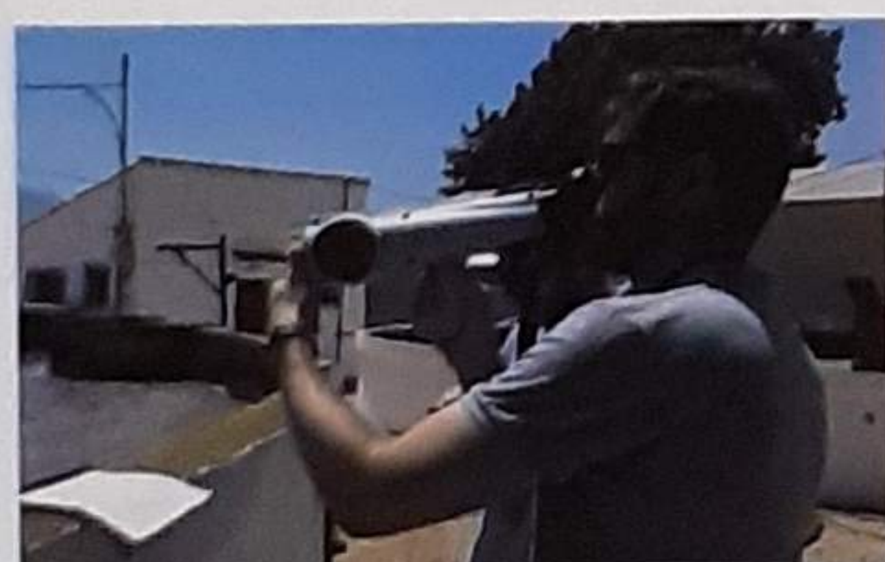
Figure 3 – Panelist measuring with Nasal Ranger ®
